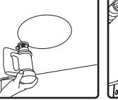
to cut hole. Hole Diameters CM42-EZs-II 165.1 mm (6.50 in) All other CMEZ, FS and BGM models daisy chaining. 266.7 mm (10.50 in)
