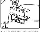
1. Unpack speaker & set 2. Use included tile bridge 3. Use Rotozip or other tool 4. Run signal wires through conduit connector, then through cover plate. Connect to ceramic terminal strip. Two + and two connectors are provided for All other CMEZ, FS and BGM models daisy chaining.
