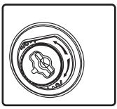
1. Select the tap position by removing the rubber plug on grille to access rotary switch. The tap switch has 2 settings: 4 ohm and 36 ohm (for 70.7V 138W/100V 276W). Select the desired setting and reinsert rubber plug. **Note:** The grille-mounted tap switch cover is keyed; be sure flat edge of plug lines up with flat edge of hole in grille.
