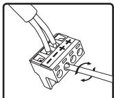
**3.** Connect signal wire to 4-pin Euroblock plug. Tighten unused terminal screws. Use inside positive and negative inputs for either voice coil or distributed systems. For daisy chaining, use outside positive and negative terminals.
