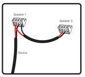
**4.** When daisy chaining, wire the outside terminals to the inside terminals of the next speaker. This step only applies to tap settings using the transformer and not when the speaker is used on bypass.
