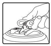
**10.** Attach the safety cable to one of the secondary holes in the hanging bracket.
