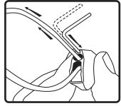
**8.** Adjust speaker hanging height with SpeedClamp™ mechanism. Pull to tighten & insert release key (small hex wrench) into SpeedClamp ™ as shown to loosen or adjust.
