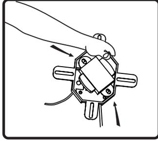
2. Remove the input module mounted onto the transformer. Unscrew to remove the transformer.
