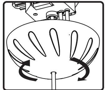
8. Move cover plate up speaker wire, begin to thread cover plate into mounting plate, leaving half an inch between cover plate and mounting surface.
