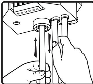
7. Set speaker height by adjusting speaker wire. Push wire through the central hole while pulling on the center slack line to shorten the speaker hanging height. Reverse to lengthen.
