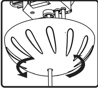
1. Remove speaker from box and unscrew the cover to reveal the mounting plate.
