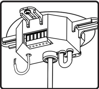
5. Connect Signal wire into terminal block
