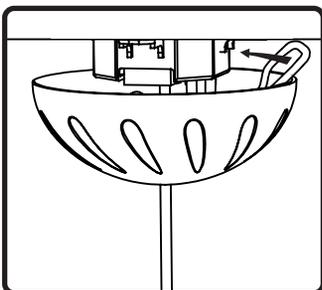
9. Excess wire can be hidden inside of cover plate by wrapping excess wire clockwise and into gap between plate and surface
