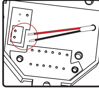
3. Un-land the red and black wires from the terminal block and splice in signal wires using wire nuts.
