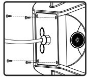
7. Install back plate and secure with included fasteners.
