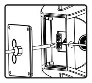
5. Run signal wires through strain relief bushing then connect to ceramic terminal strip. Two + (positive) and two - (negative) connectors are provided for daisy chaining.
