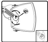
10. Aim speaker and tighten u-bracket screws. Once tightened down, place the screw caps on the screws. Done!
