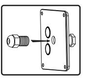
4. If being installed per EN54-24 regulations or in instances where a water tight strain relief bushing is necessary, attach the included strain relief bushing to the back plate. If it is not required, skip this step.
