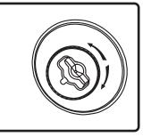
6. Select the tap position by rotating the rotary switch located on the back of the speaker to desired setting. The switch is preset to the maximum tap setting in 70.7 V mode (32W for the SM52-EZ[-WX] and 64W for the SM-82-EZ-II[-WX]).
