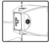
8. Select desired location for safety cable install using U-bracket mounting screw. If mounting speaker horizontally, attach safety cable to one of the vertical mounting points and vice versa.
