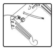
3. Mount u-bracket with clamping slots pointing upward. Securely fasten mounting bracket and safety cable to surface (user must supply fasteners). Note: The safety cable will
