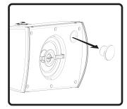
If used indoors, remove the grille and take the plug out of the port for greater bass output. Port must remain plugged to maintain IP65 rating in outdoor use.
