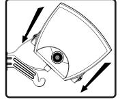
9. Tilt speaker 45° (grille up) and slide on to bracket.
