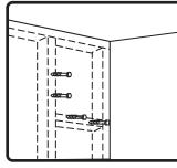
2. Choose a secure mounting surface with sufficient strength to reliably hold the speaker. The speaker may be mounted in either the vertical or the horizontal position with the same U-bracket.
